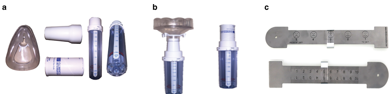
Fig. 3 a Disassembled components of the In-Check medical devices (Clement Clarke, Harlow, United Kingdom) for peak nasal inspiratory flow (PNIF) and peak oral inspiratory flow (POIF) measurements. b Assembled In-Check medical devices. c Ruler used for the measurement of the visual analog scale
